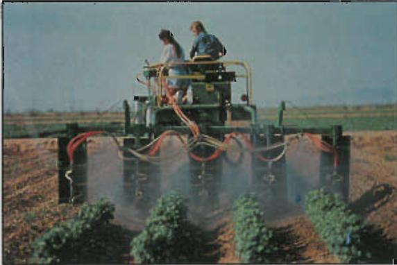
45. Thorough insecticide coverage using nozzle extensions and drops. (J. Dykinga, courtesy of USDA-ARS)
