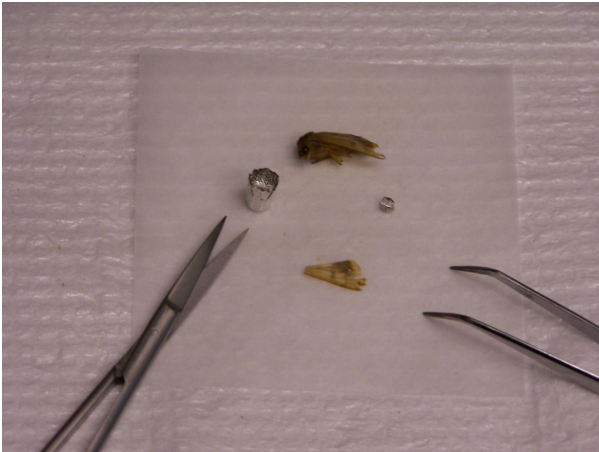
Wings cut and placed in tin capsules
